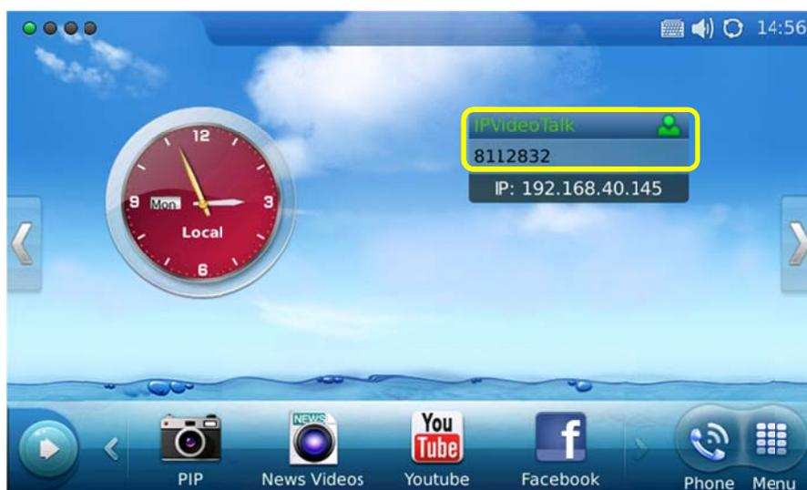
Figure 20: Making a call by select account displayed in idle screen
