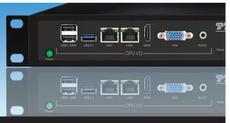
This open hardware platform, with its integrated VoIP Gateway, is ready for the operating system, IP-PBX, or Unified Communications software of your choice.
