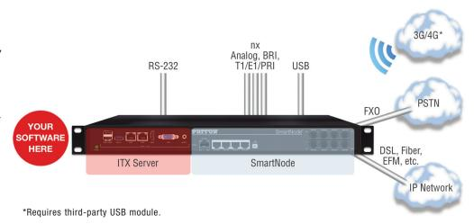
The Open Gateway Appliance is a convenient "one box" solution. With the built-in VoIP Gateway, the Open Gateway Appliance eliminates the interoperability obstacles for companies that want to keep their legacy equipment including PBXs, phones, fax equipment and POTS lines. Configuration options include a range of analog FXS/FXO and/or ISDN BRI/PRI gateways coupled with the industry standard minilTX PC board.
